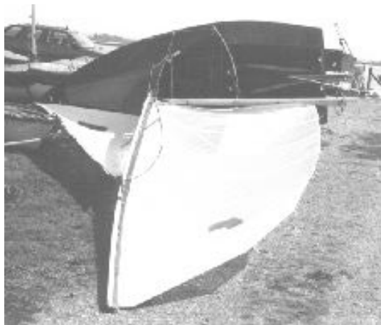
How it used to be done - Bethwaite Pine/Balsa Wing mast built around 1974 - photo Jim Champ
